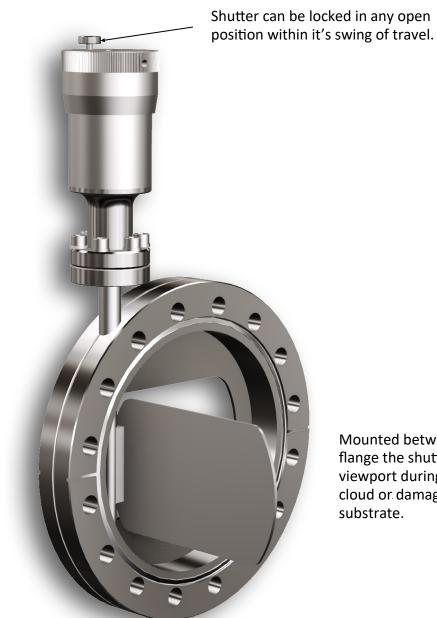
Mounted between viewport and port flange the shutter protects the viewport during processes which might cloud or damage the viewable substrate.
